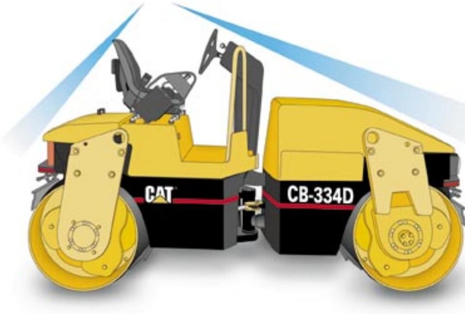
**Excellent forward visibility** allows the operator to see objects 0,6 m (2') high and 1 m (3.3') in front of the machine.
